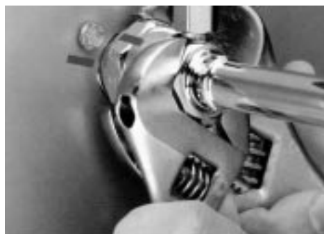
Rotate Swivel Nut \frac{1}{4} Turn More
